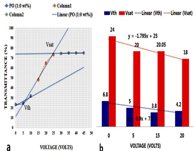
Fig. 4. Threshold voltage and saturation voltage of PDLC
