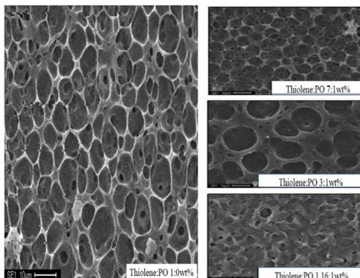
Fig. 2. SEM images of PDLC
