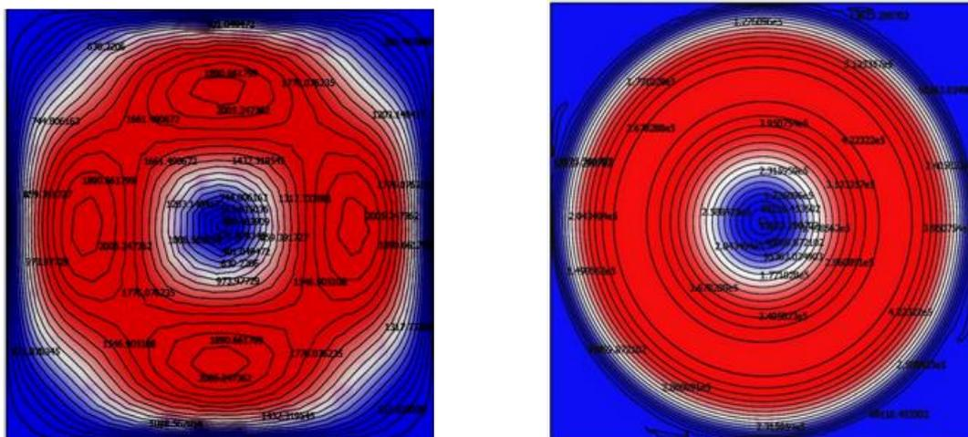
Fig. 4. Convective heat flux in the melt when the flow is only driven by buoyancy forces at various Prandtl numbers (a)  $Pr = 0.001$  and (b)  $Pr = 2$
