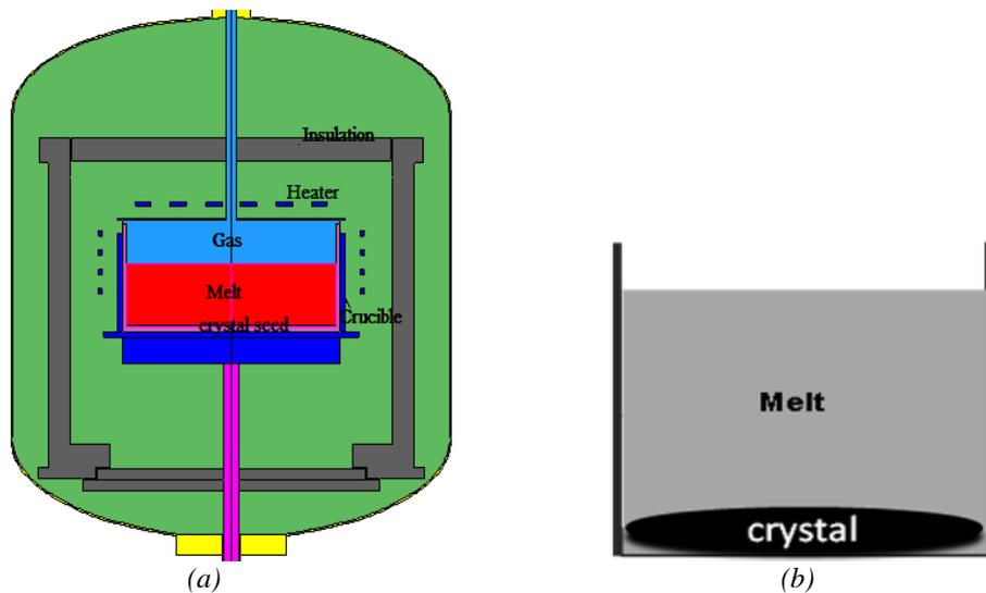
Fig. 1. (a) Schematic diagram of the directional solidification system (b) Physical system(melt)
