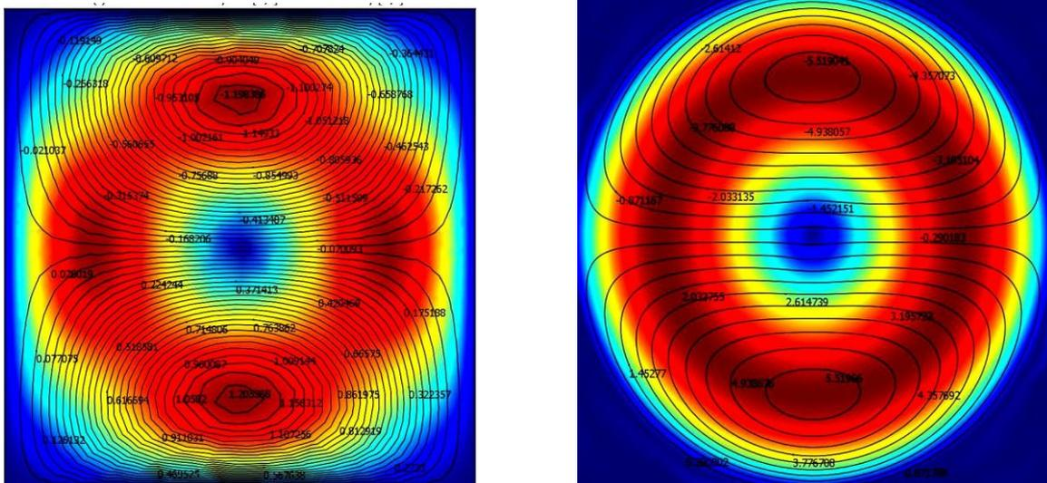
Fig. 2. Axial(X) velocities in the melt when the flow is only driven by buoyancy forces at various Prandtl numbers (a)  $Pr = 0.001$  and (b)  $Pr = 2$
