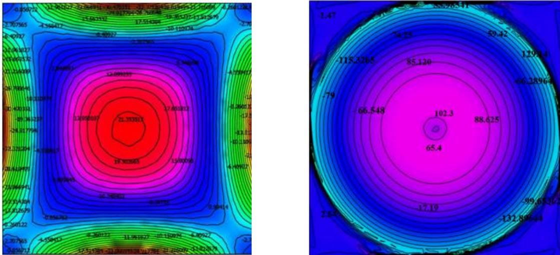
Fig. 3. Vorticity in the melt when the flow is only driven by buoyancy forces at various Prandtl numbers (a)  $Pr = 0.001$  and (b)  $Pr = 2$
