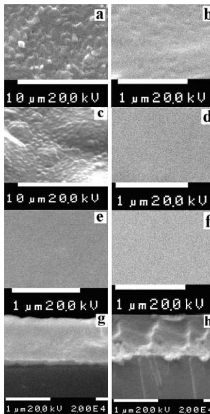
Fig.2. SEM micrographs of PMDA (a,b), ODA (c,d), PI (e,f) layers and PI cross section (g,h); (a,c,e,g) obtained without Ar plasma; (b,d,f,h) – obtained with Ar plasma assisted deposition.
