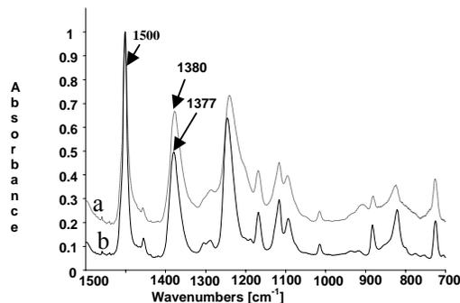
Fig.6. FTIR spectra of PI films, 500 nm thick, treated after deposition (5 min. MW and 15 min. thermal treatment): (a) obtained with an Ar plasma; (b) obtained without Ar plasma assisted deposition.
