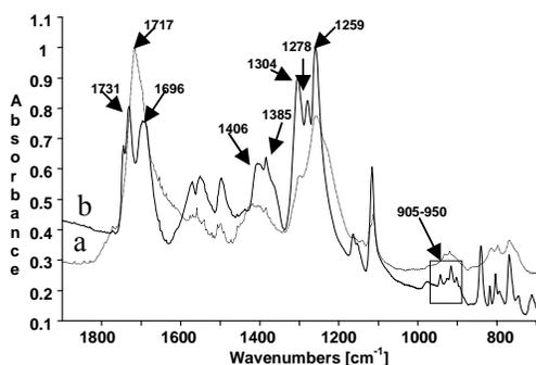
Fig.4. FTIR spectra of PMDA films, 500 nm thick: (a) obtained with Ar plasma assisted deposition; (b) obtained without Ar plasma assisted deposition.
