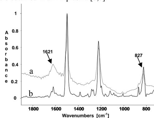
Fig.3. FTIR spectra of ODA films, 500 nm thick: (a) obtained with Ar plasma assisted deposition; (b) obtained without Ar plasma assisted deposition.
