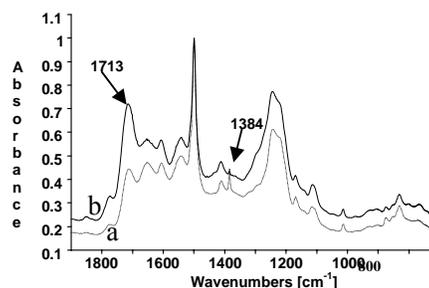
Fig. 5. FTIR spectra of PI films, 500 nm thick, untreated after deposition: (a) obtained with Ar plasma; (b) obtained without Ar plasma assisted deposition.
