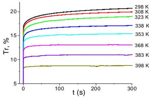
Fig. 4. Kinetics of thermal PD erasing at various temperatures
