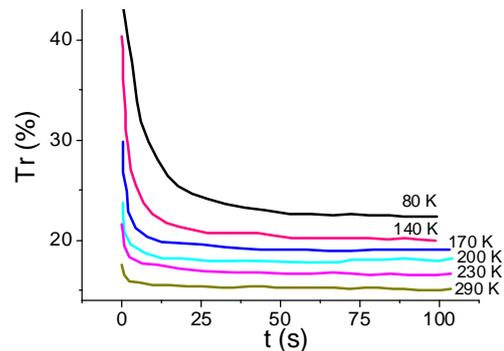
Fig. 1. PD kinetics (transmission) in  $As_{20}Se_{80}$  layers at different temperatures
