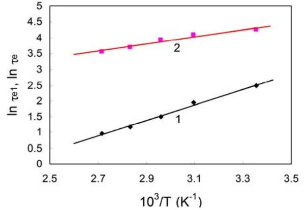
Fig. 6. Temperature dependences of erasing times: 1 - for transient ( $\tau_{e1}$ ) and 2 - for metastable PD component ( $\tau_e$ )
