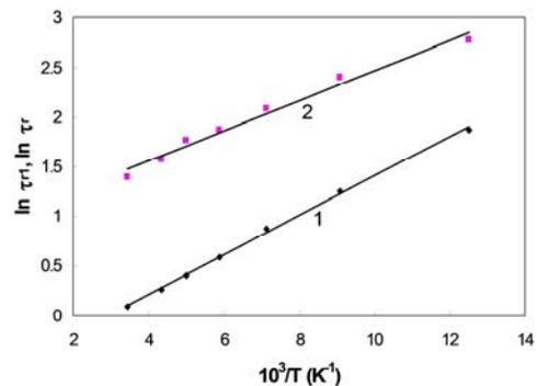
Fig. 3. Temperature dependences of recording times: 1 - for transient ( $\tau_{r1}$ ) and 2 - for metastable PD component ( $\tau$ )
