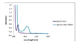
Fig. 10. UV-Vis spectra of the studied gels with oregano (gel O) and curcumin (gel Cu)
