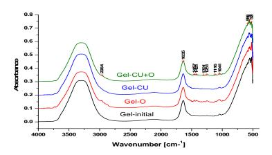
Fig. 9. IR absorption spectra for gel samples containing essential oil of oregano (Gel-O) and curcumin extract (Gel-Cu)
