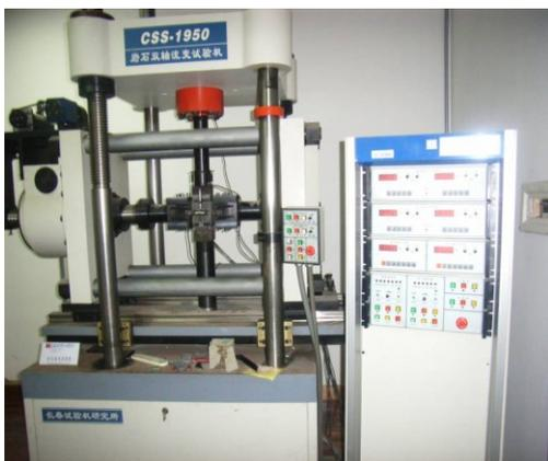
Fig. 1 CSS-1950 rock rheology biaxial testing machine (image by Zhang et al.)
