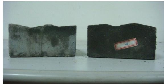
Fig. 2 The steel model of Barton's standard profiles and the specimen (image by Zhang et al.)
