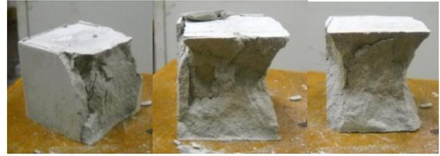
Fig. 3 Failure specimens during uniaxial compression tests.
