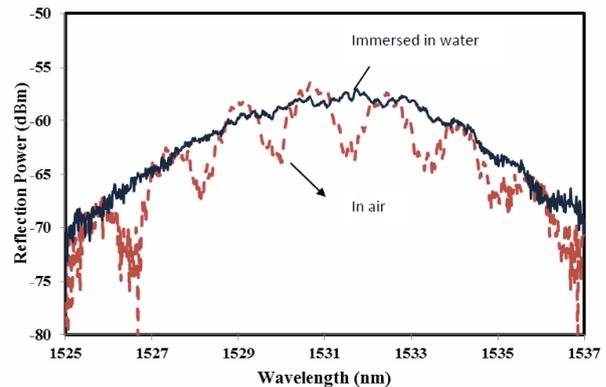
Fig. 4: Output spectra obtained as the micro-ball lens is immersed in air and water
