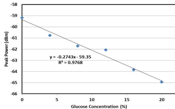
Fig. 5: Peak output power of the micro-ball lensed fiber for different glucose concentration
