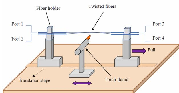
Fig. 1: Fabrication setup for microfiber coupler
