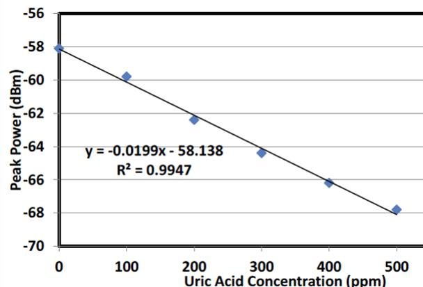
Fig. 6: Peak output power of the micro-ball lensed fiber for different uric acid concentration
