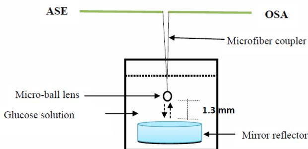
Fig. 3. The schematic diagram of the proposed glucose sensor.
