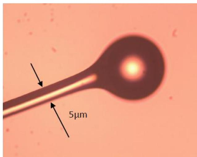
Fig. 2: Microscope image for the micro-ball lens fabricated at the cleaved tip of MFC
