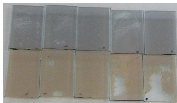
Fig. 2. Peeling of the gold layer deposited directly on the glass plates of the same batch after overnight contact with ethanol. Up: samples of the P(8) batch; down: samples of P(5) batch. The black sign on the glass back comes from the initial mark of the plates.
