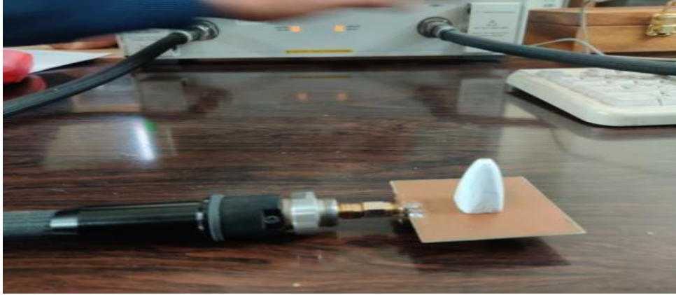
Fig. 7. Fabricated conical -DRA under measurement (color online)
