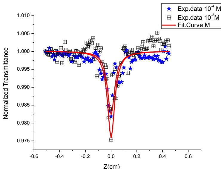
Fig. 4. Open aperture z-scan data of MPTC in chloroform at two concentrations of concentrations of 10<sup>-3</sup>M and 10<sup>-4</sup>M (color online)
