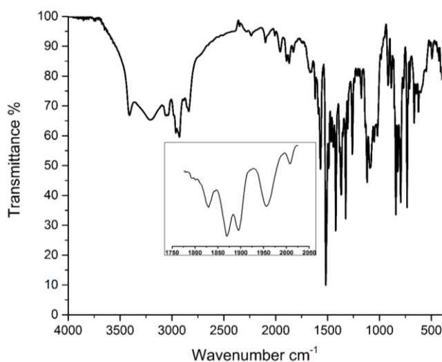
Fig. 3 FTIR spectrum of MPTC as KB disc
