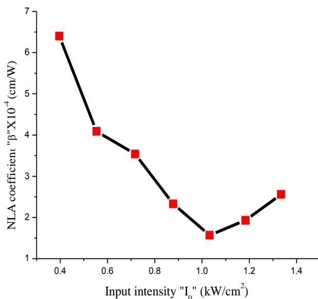
Fig. 5. The nonlinear absorption coefficient  $\beta$  versus on-axis input intensity  $I_0$  of MPTC in chloroform (color online)
