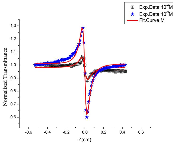
Fig. 6. Pure (C/O) z-scan data of MPTC in chloroform at two concentrations of concentrations of  $10^{-3}M$  and  $10^{-4}M$  (color online)
