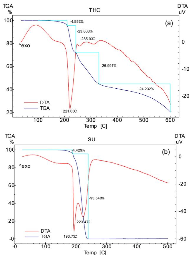
Fig. 4 DTA /TGA curves of thiamine hydrochloride (a) and succinic acid (b) (color online)
