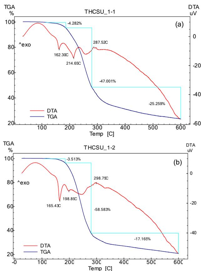
Fig. 5. DTA/TGA curves of THCSU samples (color online)
