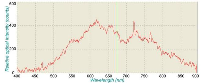
Fig. 6. Optical spectrum observed at  $V_{sub} = 48$  V,  $V_d = V_s = 0$  V, and floating gate. In this case,  $V_{sub}$  is equivalent to the reverse bias of the “ $P^+$  Source/Drain to N-Substrate” junction diode
