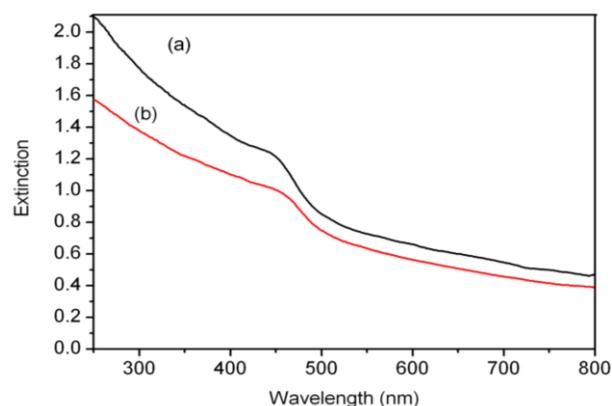
Fig. 6. UV-Vis extinction spectra of CdS doped silica nanomaterials (a) sample 2; (b) sample 3.
