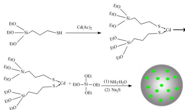
*Scheme 1 a scheme diagram to illustrate preparation process of hybrid silica materials.*
