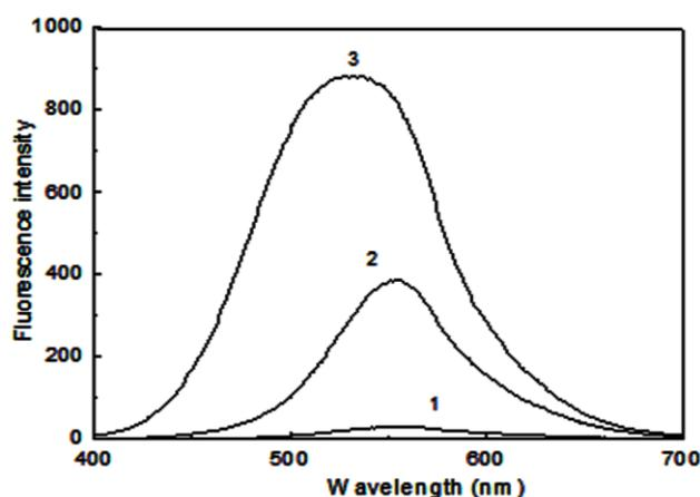
Fig. 5. Fluorescence emission spectra of CdS doped silica nanomaterials: (1) sample 1; (2) sample 2; (3) sample 3.
