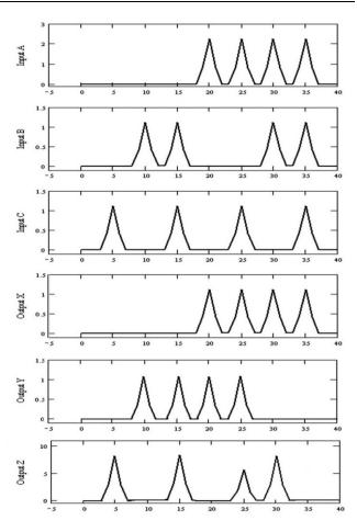
Fig. 4. Logical simulation result [x- axis: time (ps) and y-axis: power (dBm)].
