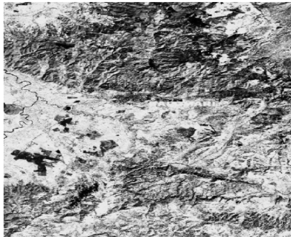
Fig. 2. PCA (4/5/3) analysis for Baia Mare mining area on satellite Landsat ETM 22/08/2000 image.
