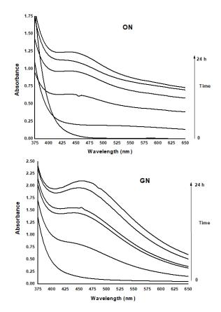
Fig. 1. The bioreduction of  $Ag^+$  to  $Ag^0$  by using peels' extracts of oranges (ON) and grapefruits (GN)
