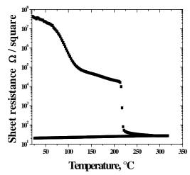
Fig.4. Temperature dependent sheet resistance measurements for the  $Ge_{13}Te_{67}$   $Ga_{20}$  film.
