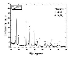
Fig. 3. Diffractogramme of the  $Ge_{13}Te_{67}Ga_{20}$  film annealed at 250°C.
