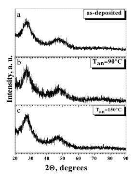
Fig. 2. XRD spectra of the  $Ge_{13}Te_{67}Ga_{20}$  alloy as deposited curve (a), after annealing at 90°C (curve b) and 150°C (curve c), respectively.
