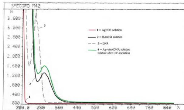
Fig.2. Absorption spectra of the  $\text{AgNO}_3$ ,  $\text{HAuCl}_4$  solutions and Au-Ag-DNA solution mixture after 30 min UV-irradiation (at UV lamp).
