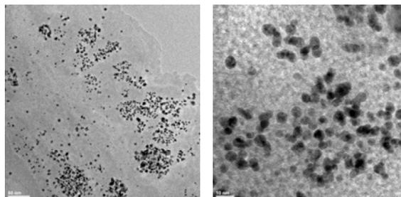
Fig. 10. TEM images of the Au-Ag-DNA alloy particles after 3 hours of UV-photoirradiation
