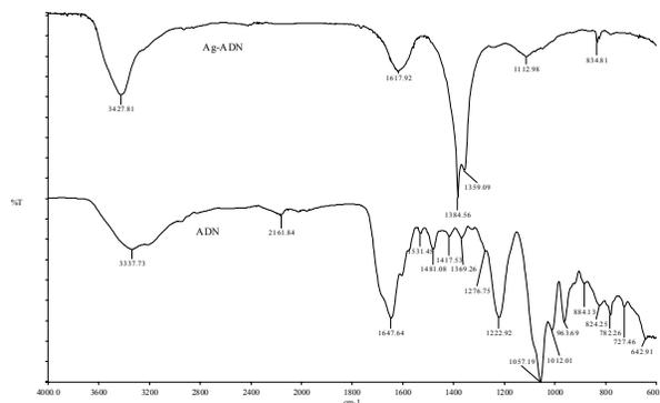
Fig. 5. FTIR spectra of DNA and Ag-DNA complex
