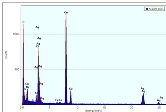
Fig. 11. EDX image of Ag-DNA nanoparticles
