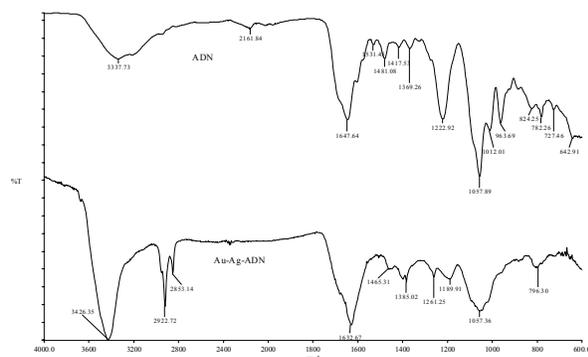
Fig. 7. FTIR spectra of DNA and Au-Ag-DNA complex
