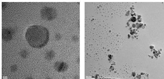
Fig. 8. TEM images of the Ag-DNA alloy particles after 3 hours of UV-photoirradiation
