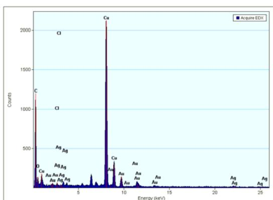
Fig. 13. EDX image of Au-Ag-DNA nanoparticles
