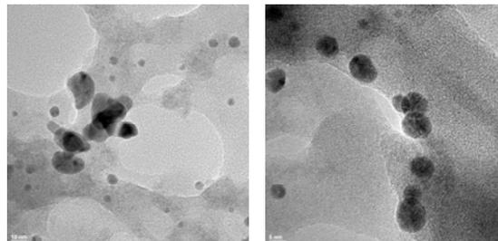
Fig. 9. TEM images of the Au-DNA alloy particles after 3 hours of UV-photoirradiation
