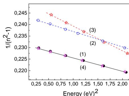
Fig. 2. Dispersion of the refractive index ( $n$ ) according to the Wemple-DiDomenico model for the  $\text{Ge}_{10.7}\text{As}_{21.65}\text{S}_{67.65}$  film ( $d \approx 700$  nm): (1) fresh, (2) ill., (3) ann., (4) ill. after annealing.
