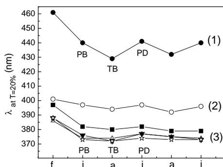
Fig. 4. Photo- and thermally-induced changes in films of  $Ge_{11.2}As_{18}S_{70.8}$  glass with different thicknesses in the illuminated (i) and annealed (a) states.
