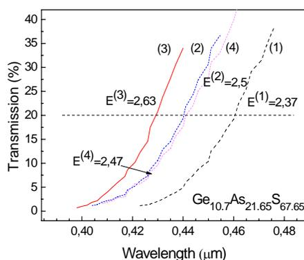
Fig. 1. Transmission curves of the film with  $d \sim 700$  nm in different states: (1) fresh, (2) ill., (3) ann., (4) ill. after annealing. The calculated values of the optical band gap in eV are as indicated.
