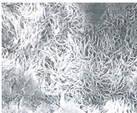
Fig. 2. SEM micrograph of \text{CdS}_{0.70}\text{Se}_{0.30} film
