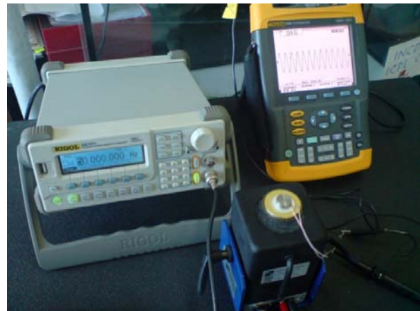
Fig. 6. SHOP MODE system for creating vibrations that operates in frequency range: 5Hz - 1kHz.
