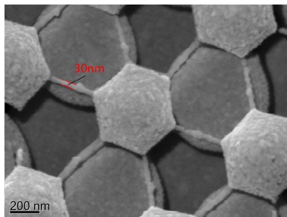
Fig. 5. SEM image of a plasma treated NSL double-layer mask made from 1000 nm diameter PS spheres. A 30 nm Ag film was deposited prior to SEM inspection.
