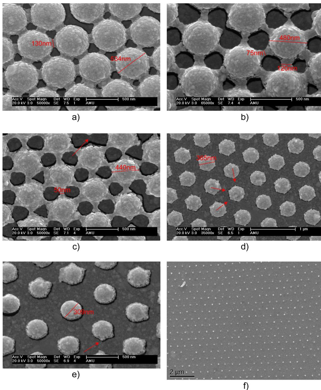
Fig. 2. SEM images of a 600 nm diameter PS bead mask treated for 3 (a), 4 (b), 5 (c), 6 (d), 7 (e) and 14 min (f) in a 50 W air plasma. The samples were covered with 30 nm Ag to improve contrasts, resulting in the grainy surface morphology.
