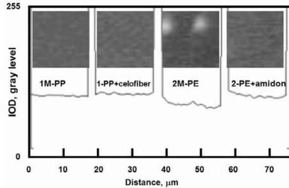
Fig. 2. IOD profiles for the typical samples of PP, PP with 20% Celofiber, PE and PE with Amidon in magnified zone areas of size  $\sim 16 \times 16 \mu\text{m}$ .
