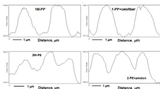
Fig. 3. Typical detailed profile plots for single particles details of the 4 dielectric materials types investigated. The 1-PP-celofiber sample particles were calibrated by SEM images to give an approximate height of 250 nm for the spheroids.
