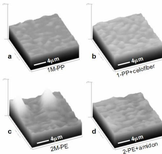
Fig.1. DELI 3D zoomed images of 4 samples areas : a.) PP, b.) PP with 20% Celofiber, c.) PE and d.) PE with Amidon in magnified zone areas of size  $\sim 16 \times 16 \mu\text{m}$ .
