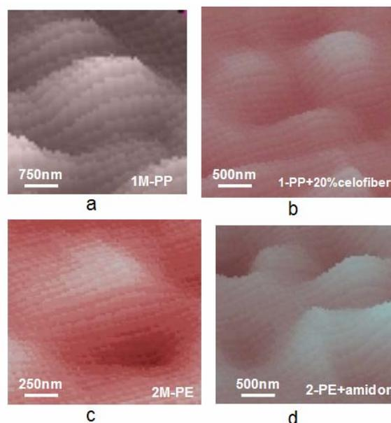
Fig. 4. DELI processed micrographs by Image Processing, giving 3D perspective of the nano-structural details at the highest magnification: a) for 1M-PP; b) for 1-PP+Celofiber; c) for 2M-PE; d) for 2-PE+Amidon.
