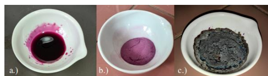
Fig.1: a.) Co(NO 3 ) 2 ·6H 2 O – diol solution; b.) Powder – isolated complex combination; c.) Powder – burning of the complex combination
