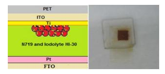
Fig. 1. Schematic of DSSC and new DSSC (color online)
