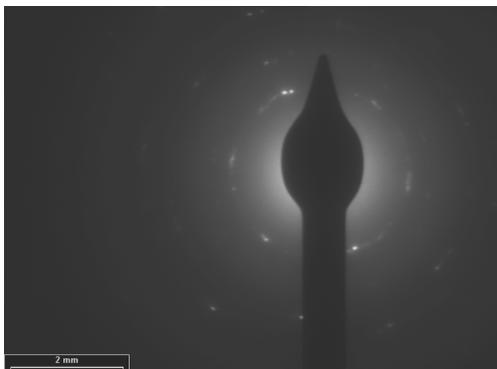
Fig. 2a. SAED image of the CaPT0 ceramic sintered at 1000°C.
