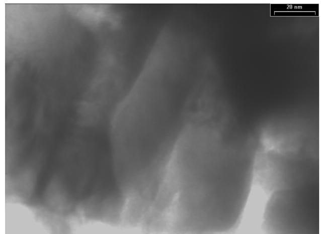
Fig. 1f. HRTEM images in CaPT0 material sintered at 1030°C. Scale bar: 20nm
