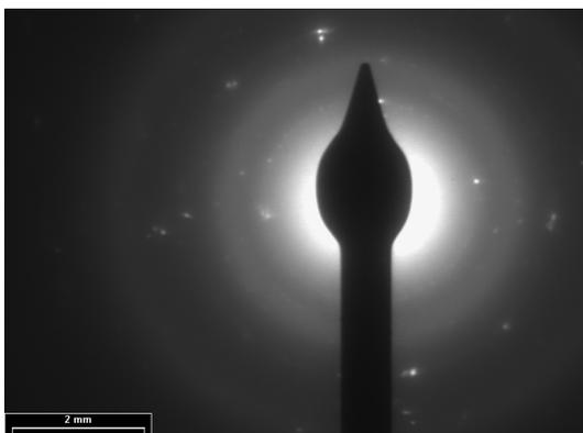
Fig. 2b. SAED image of the CaPT0 ceramic sintered at 1010°C
