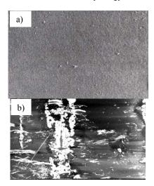
Fig. 5 Surface morphology of an as-deposited boron film (a) and a layer treated at 1200 °C for 180 s.
