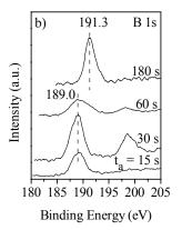
Fig. 4. Evolution of N 1s (a) and B 1s (b) XPS spectra with the annealing time of films obtained at 1400° C.
