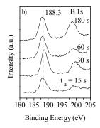
Fig. 3. N 1s (a) and B 1s (b) XPS spectra of films formed at 800 °C for different t<sub>a</sub>.
