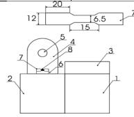
Fig. 1. Schematics of the RTP system: 1- system electronics, 2-vacuum system, 3-operation block, 4- vacuum camera, 5 - windows, 6- electrodes, 7-heater(dimensions in mm), 8- substrate.
