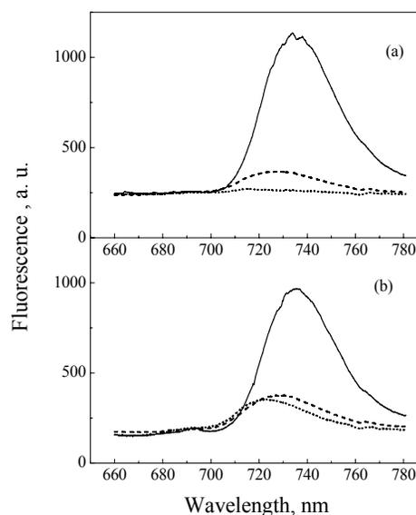
Fig. 1. 77 K fluorescence emission spectra of PSI particles under high light treatment: illuminated for 0 min (solid line), 60 min (dashed line) and 120 min (short dashed line) in: (a) control PSI particles; (b) histidine-containing PSI particles.
