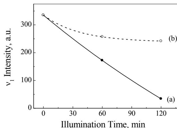
Fig. 3. Dependence of  $\nu_1$  band intensity on the time of illumination of lutein molecules: (a) in control PSI particles; (b) in histidine-containing PSI particles.
