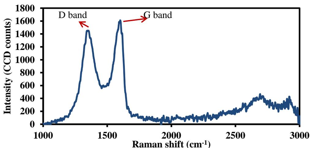
Fig. 2: Raman spectrum of graphene oxide.
