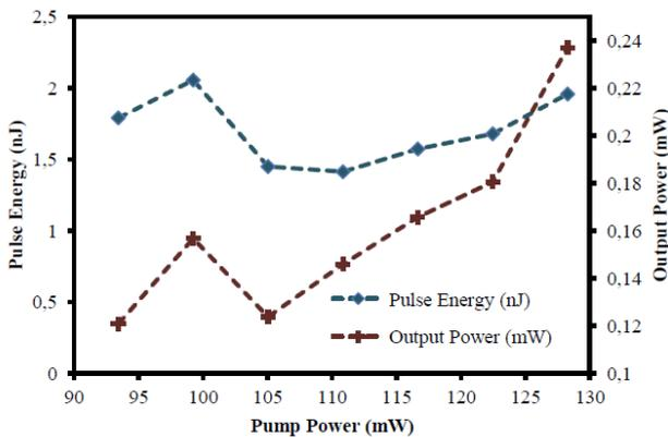
Fig. 7: Pulse energy and output power as a function of pump power
