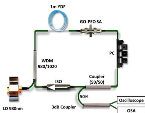
Fig. 3: Schematic configuration of the Q-switched YDFL.
