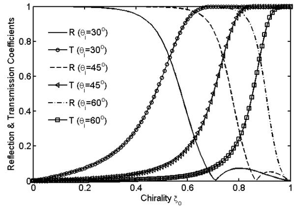
Fig. 3. Reflection and Transmission coefficients of chiral nihility slab versus the chirality parameter for different values of the incident angles.
