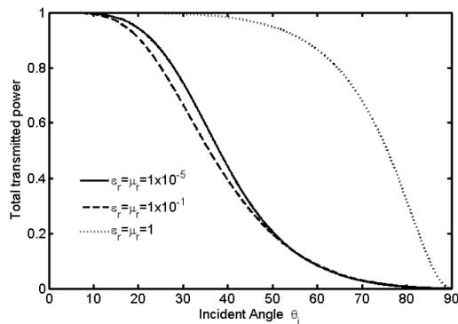
Fig. 5. Total transmitted power versus incident angle for three different values of  $\epsilon_r$  and  $\mu_r$ . ( $\xi_0 = 0.25$ ,  $f = 10$  GHz,  $d = 5$  mm).
