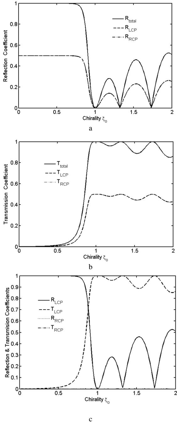
Fig. 2 (a) Reflection (b) Transmission coefficients for perpendicularly polarized incident wave (c) Reflection and transmission coefficients for LCP incident wave ( $\theta_i = 60^\circ$ ).
