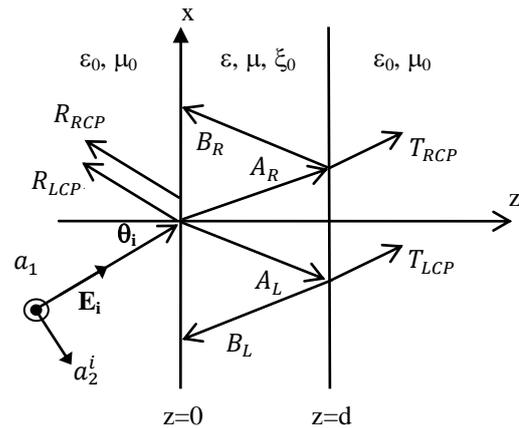
Fig. 1. The configuration of an infinitely long chiral nihility slab of thickness  $d$  located between  $z=0$  and  $z=d$ .
