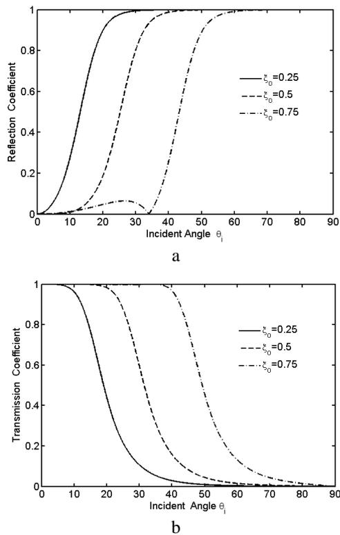
Fig. 4. (a) Reflection and (b) Transmission coefficients of chiral nihility slab versus the angle of incidence for different values of the chirality parameter.
