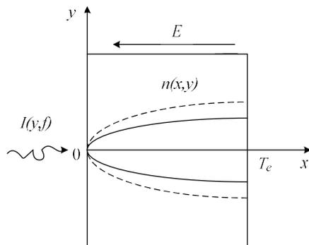
Fig. 3. Schematic diagram of electron transport within a GaN photocathode. Solid lines represent electron transport with a constant built-in electric field; Dashed lines represent electron transport without this electric field
