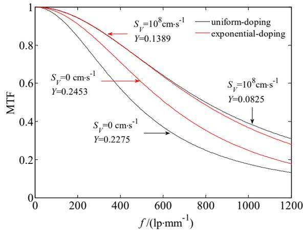
Fig. 7. MTF of the exponential-doping and uniform-doping GaN photocathodes for  $S_V = 0$  and  $10^8 \text{ cm} \cdot \text{s}^{-1}$ , and the corresponding values of  $Y$ , when  $T_e = 0.6 \mu\text{m}$ ,  $L_d = 1.0 \mu\text{m}$ , and  $\alpha = 4 \times 10^4 \text{ cm}^{-1}$
