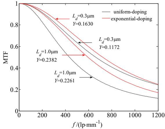
Fig. 4. MTF of the exponential-doping and uniform-doping GaN photocathodes for  $L_d=0.3 \mu\text{m}$  and  $1.0 \mu\text{m}$  and the corresponding values of  $Y$  when  $T_e = 0.6 \mu\text{m}$ ,  $\alpha = 4 \times 10^4 \text{cm}^{-1}$  and  $S_V = 0$
