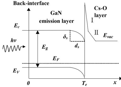
Fig. 1. Band structure diagram of a transmission-mode uniform-doping GaN photocathode.  $E_c$  is the conduction-band minimum,  $E_v$  is the valence-band maximum,  $E_g$  is the band gap,  $E_F$  is the Fermi level,  $\delta_s$  and  $d_s$  are the height and width of the bent-band region, respectively, and  $E_{vac}$  is the vacuum level.
