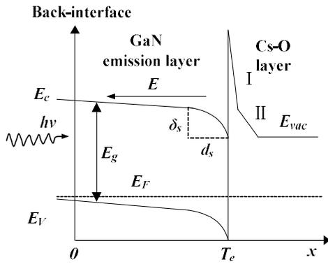
Fig. 2. Band structure diagram of a transmission-mode exponential-doping GaN photocathode.  $E$  is the strength of built-in electric field
