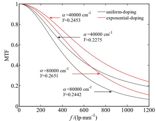
Fig. 6. MTF of the exponential-doping and uniform-doping GaN photocathodes for  $\alpha = 40000 \text{cm}^{-1}$  and  $80000 \text{cm}^{-1}$  and the corresponding values of  $Y$ , when  $T_e = 0.6 \mu\text{m}$ ,  $L_d = 1.0 \mu\text{m}$  and  $S_V = 0$
