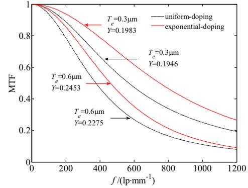
Fig. 5. MTF of the exponential-doping and uniform-doping GaN photocathodes for  $T_e = 0.3 \mu\text{m}$  and  $0.6 \mu\text{m}$  and the corresponding values of  $Y$ , when  $L_d = 1.0 \mu\text{m}$ ,  $\alpha = 4 \times 10^4 \text{cm}^{-1}$ , and  $S_V = 0$ .
