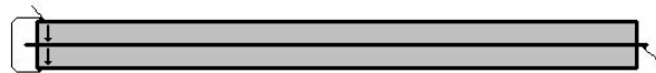
Fig. 1 The parallel bimorph. The arrows indicate the polarization directions of the discs.
