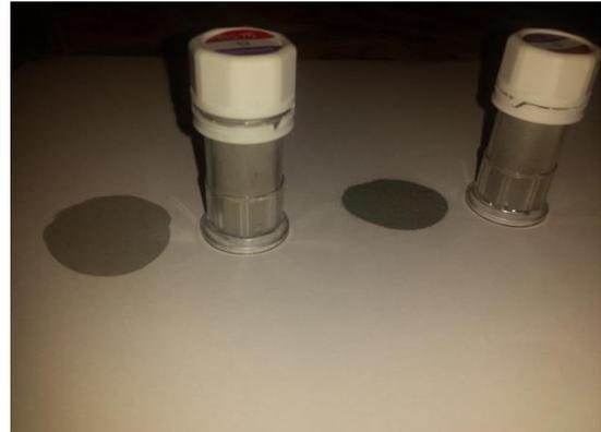
Fig. 6. Co-Cr alloy powder with diameter of granules <math><30 \mu\text{m}</math> and <math>>50 \mu\text{m}</math> respectively
