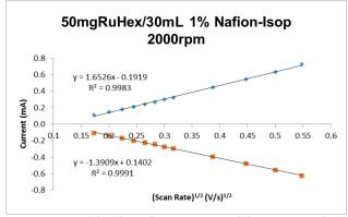
Fig. 7. Peak height vs the square root of the scan rate of isopropanol diluted 50mg RuHex electrode
