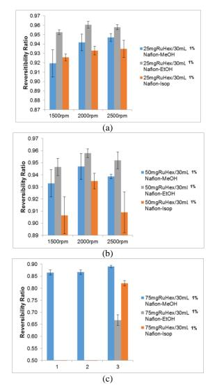
Fig. 4. Comparison of reversibility ratios for 25mg RuHex (a), 50mg RuHex (b), and 75mg RuHex (c) modified electrodes
