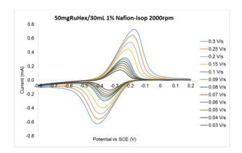
Fig. 6. Multiple scan rate voltammogram for isopropanol-diluted 50mg RuHex electrode
