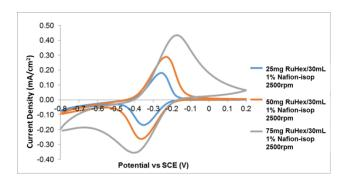
Fig. 1. Comparison of isopropanol diluted 25 mg RuHex, 50 mg RuHex, and 75 mg RuHex electrodes
