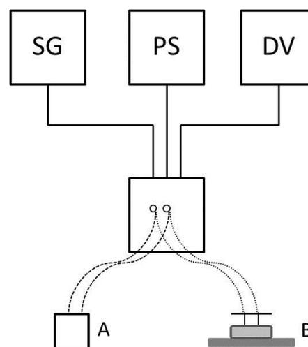
Fig. 1. Block-scheme of the electric bio-impedance measurements unit, consisting of SG-signal generator, PS – power supply, DV- digital voltmeter, A - cuvette with a platinum electrode for a liquid media, and B - needle-shaped electrodes for solid media measurements of a submerged type fixed on a common base
