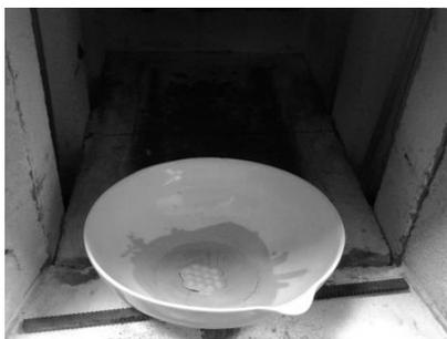
Fig.3. Drying of the biocomposite mixture HAP/Ti in the furnace after milling
