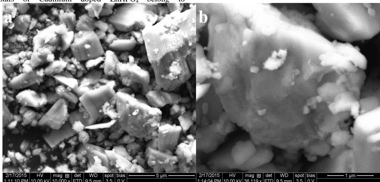
Fig. 2 (a): SEM image of cadmium doped ZnHPO<sub>4</sub> crystal (b) Magnified SEM image
