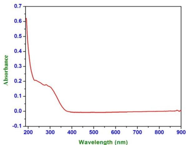
Fig. 4 UV absorption of Cadmium doped  $\text{ZnHPO}_4$
