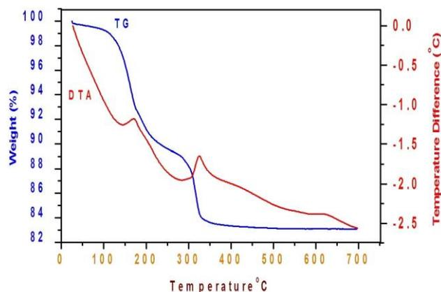
Fig. 5 Thermogram showing simultaneous recording of TG and DTA curves for Cadmium doped ZnHPO<sub>4</sub>
