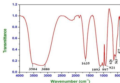
Fig. 3 FTIR Spectrum of Cadmium doped ZnHPO<sub>4</sub>
