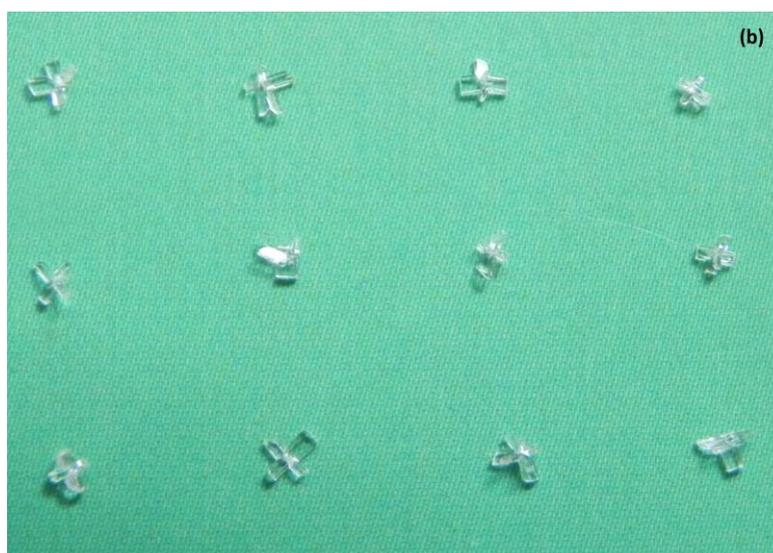
Fig. 1 (a) cadmium doped  $\text{ZnHPO}_4$  crystals grown in gel medium & (b) Morphology of cadmium doped  $\text{ZnHPO}_4$  crystals
