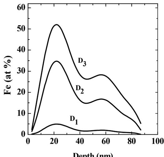
Fig. 1.  $\text{Fe}^+$  implantation profiles for the first set of samples, simulated by SRIM.
