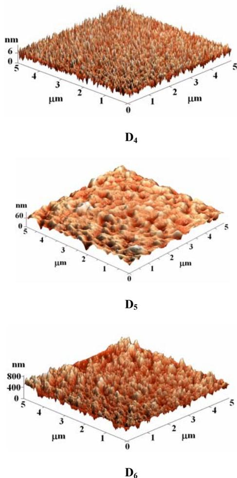
Fig. 6. AFM images of as-implanted ( $D_4$ ), and annealed ( $D_5$  and  $D_6$ ) samples
