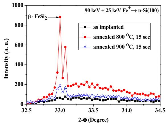
Fig. 3. XRD spectra of Fe implanted and annealed Si samples ( $D_4$ ,  $D_5$  and  $D_6$ ).
