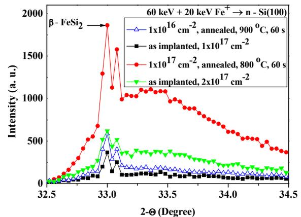
Fig. 2. XRD spectra of Fe samples implanted in Si with doses D<sub>1</sub>, D<sub>2</sub> and D<sub>3</sub> and annealed.
