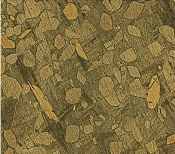
*Fig. 7. Ti6Al4V Titanium alloy, vacuum hardened at 1020°C and annealed at 500°C for 30 minutes, 1000:1*
