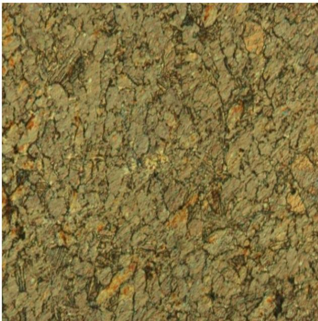
Fig. 3. Ti6Al4V Titanium alloy, delivery state, 1000:1
