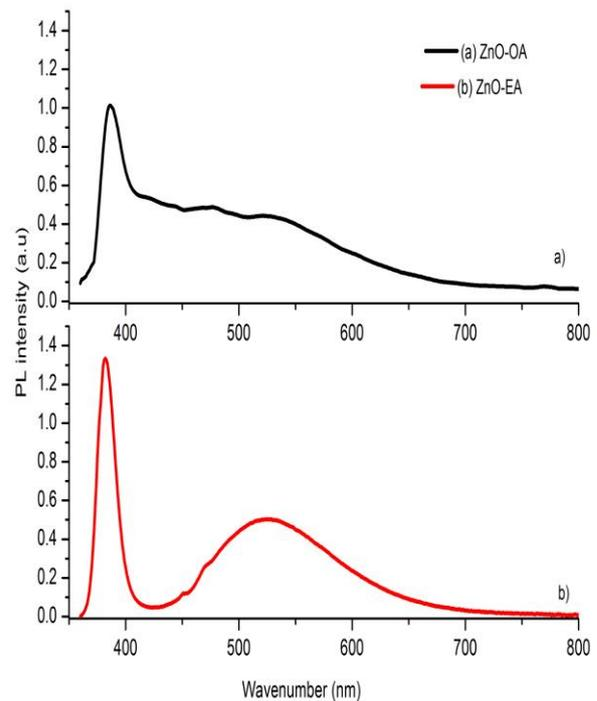
Fig.4. PL spectra of a) ZnO-OA and b) ZnO-EA powders
