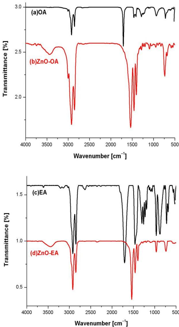
Fig.3. FTIR spectra of a) ZnO-OA and b) ZnO-EA powders
