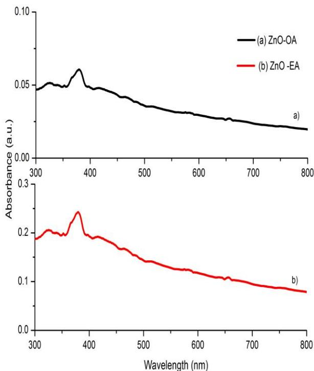
Fig.5. UV-VIS spectra of a) ZnO-OA and b) ZnO-EA powders
