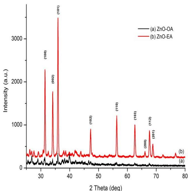
Fig.2. XRD pattern of a) ZnO-OA and b) ZnO-EA powders
