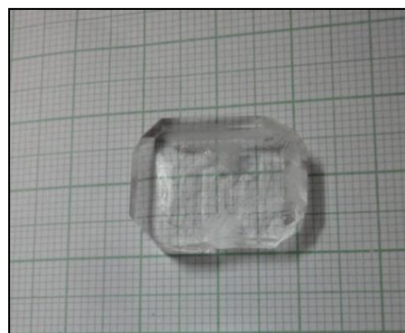
Fig.1. Photograph of the as grown crystal of ADP-MA.
