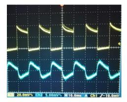
Fig. 8. Optical switching effect: pump beam (upper trace) and probe beam (lower trace) (color online)
