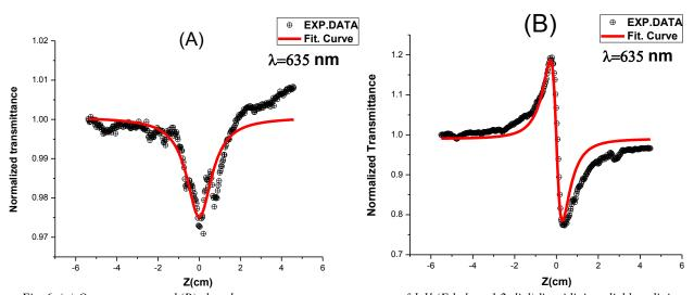
Fig. 6. (a) Open aperture and (B) closed aperture z-scan measurements of 1,1'-(Ethylene-1,2-diyl)dipyridinium dichlorodinitratocuprate(II) in DMSO with concentration of  $10^{-3}M$ , at  $\lambda = 635$ nm. The solid line is a fit of the experimental data (color online)
