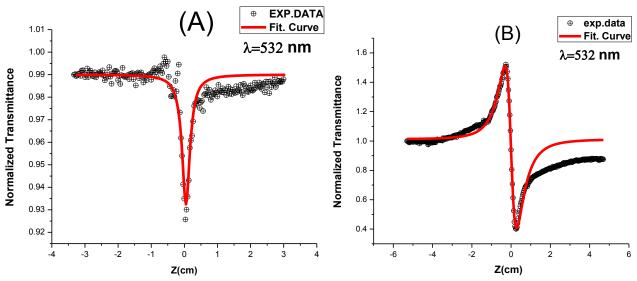
Fig. 7. Normalized transmittance (close aperture) of 1,1'-(Ethylene-1,2-diyl)dipyridinium dichlorodinitratocuprate(II) in DMSO with concentration of  $10^{-3}M$  at two laser wavelengths,  $\lambda = 635$  and  $\lambda = 532$  nm. The solid line is a fit of the experimental data (color online)
