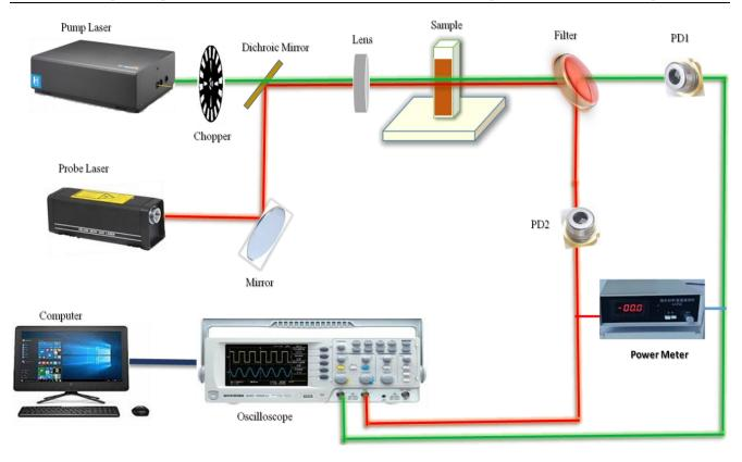
Fig. 5. The pump-probe experimental setup for optical switching measurements (color online)
