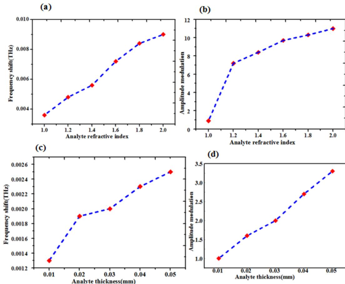
Fig. 3. (a) Frequency shift versus analyte refractive index, (b) Amplitude modulation versus analyte refractive index at a top layer thickness of 50 $\mu\text{m}$ , (c) (d) Frequency shift and amplitude modulation versus analyte thickness (color online)
