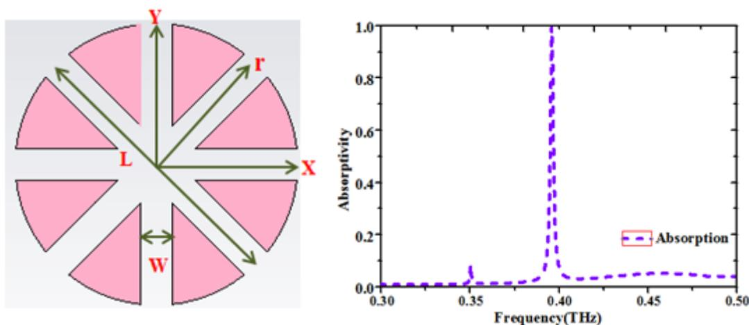
Fig.1. (a). Geometrical parameters of the metamaterial unit cell ( $r=0.16\text{mm}$ ,  $l=0.32\text{mm}$ ,  $w=0.036\text{mm}$ ), 1(b) Absorption curve for the proposed absorber (color online)
