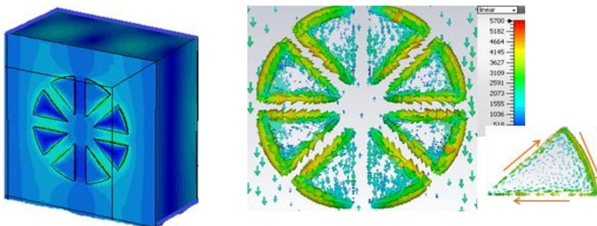
Fig.4. (a).Distributions of the magnetic field for the proposed terahertz sensor at a frequency of 0.3956 THz, (b) Surface current distribution and direction of the current flow (color online)
