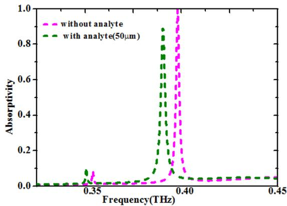
Fig.2. (a) Simulated absorption curves with a 50- $\mu\text{m}$ -thick analyte and without analyte (color online)
