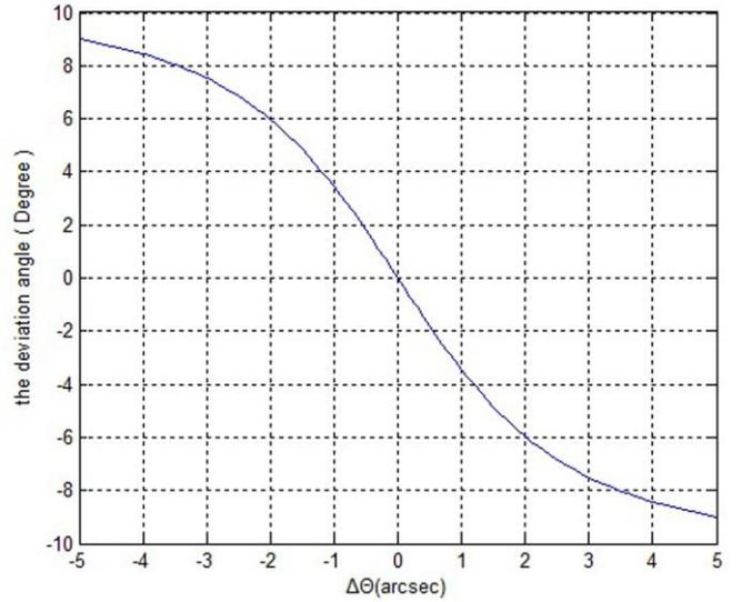
Fig.2. the deviation angle  $\theta_{out}$  changed with the  $\Delta\theta$  caused by the refraction in sample. a small deviation of the X-ray incident angle is amplified many times by the crystal diffraction.
