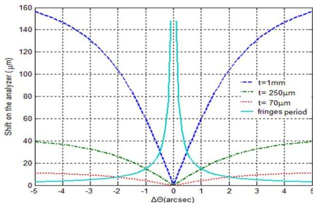
Fig.3. the shift distance of exit point for different thickness of the analyzer comparing with the fringes period. Calculations conditions are: the Laue-case Si 220 diffraction,  $P=1$ ,  $\lambda=0.07$  nm.
