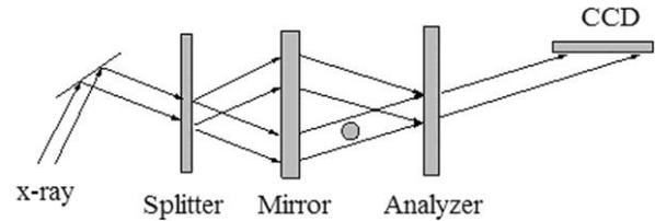
Fig.1 X-ray interferometry method based on the crystallography. The LLL interferometer consists of three Si blades Splitter, Mirror, Analyzer.
