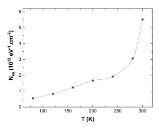
Fig. 7. N<sub>ss</sub>-T graph of Au/n-GaAs contacts
