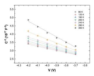
Fig. 5. C<sup>-2</sup>-V graph of Au/n-GaAs contacts (color online)
