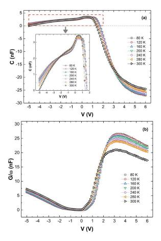
Fig. 2. (a) C-V graph (b) G/ω-V graph of Au/n-GaAs contacts (color online)
