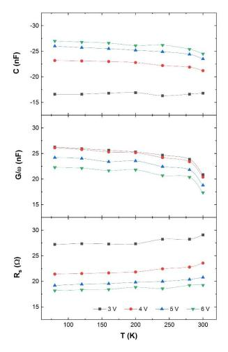
Fig. 4. C-T, G/ $\omega$ -T and R<sub>s</sub>-T graphs of Au/n-GaAs contacts (color online)
