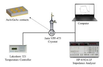
Fig. 1. Schematic diagram of Au/n-GaAs contacts and the measurement system (color online)
