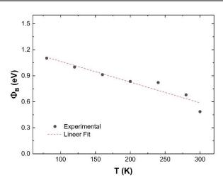
Fig. 6.  $\Phi_B$ -T graph of Au/n-GaAs contacts (color online)
