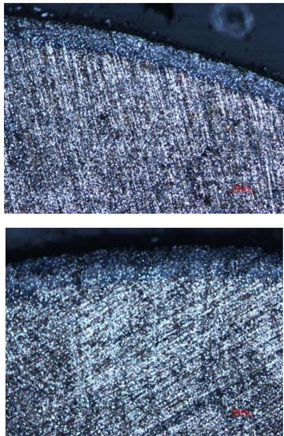
Fig. 4 - Nitrocarburized layers, El CrW2 electrode coating, X 200, Nital etch
