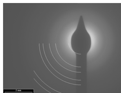
Fig. 10. SAED image for \text{Zn}_{0.75}\text{Cd}_{0.25}\text{S} sample synthesized in water – acetone 1/1 environment.
