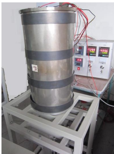
Fig. 1. The single crystal grown furnace using vertical Bridgman method.
