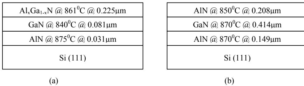
Fig. 1. Cross-section structures of (a) Al x Ga 1-x N and (b) AlN cap layers on GaN/AlN/Si sample.
