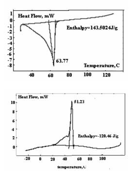
Fig. 1. Thermograms of Prunus domestica soft wax: (a) from the heating program, (b) from the cooling program
