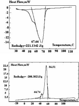
Fig. 2. Thermograms of Prunus cerasifera hard wax: (a) from the heating program, (b) from the cooling program
